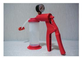
Figure 6 Using a vacuum pump to demonstrate water boiling below 100 °C under reduced pressure
